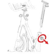
6. Pull down on the seat slider locking pin then slide the seat assembly onto the seat post installed in Step 3, tightening the fore/aft adjustment knob to lock the seat slider into place.
