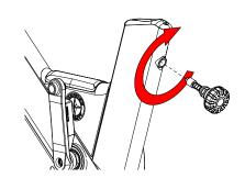
Slide the seat post into the frame by loosening the seat post pop pin, then pulling outwards on the pin while sliding the seat into the frame.
